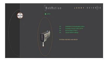
If the XENAX® servo controller does not recognize a LINAX® or ELAX® linear motor axis or a ROTAX® rotary axis, XENAX® assumes a connection with third party motor. Instead of "Go Pos 0" WebMotion® offers
