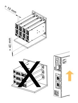
When operating with a power supply motor above 60VDC, the XENAX® Servo controller must be mounted in an electrical control cabinet and the XENAX® Servo controller must be connected to protective earth using the shielding clamp (Art. No. 130.09.00) for motor cable.
