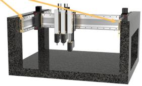
The arrangement of the two linear motor axes
