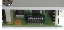
DIP switch 2 ON Logic supply ON, firmware recorder is being deleted, wait until "F" on display, logic supply off, DIP switch 2 OFF
