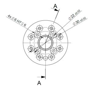
Centering rings for boreholes Ø6H7x1 in Pitch circle diameter 30
