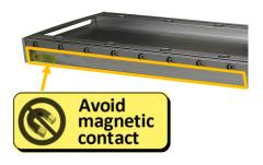
Incorrect handling of the linear motor axes with optical measuring system can scratch the glass scale and thus lead to errors. Keep it clean and do not touch it directly with your hand. To clean the optical measuring system, use a lint-free cloth and cleaning spirit.
