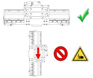
For linear motors with cover (Lxe) is a risk to bend the steel cover plate. It is to be careful not to carry the linear motor on the cover plate.
